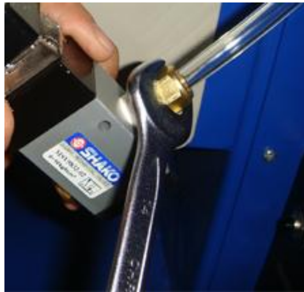
◆ Use the combination wrenches to lock the copper nut to the copper fitting.
