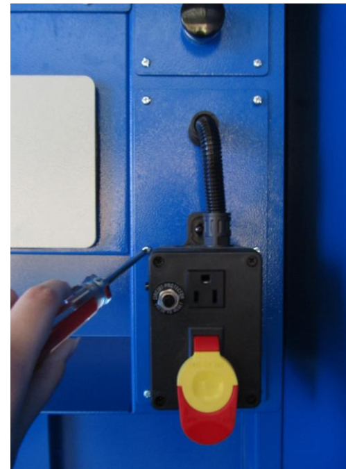
◆ Use the screwdriver with the Phillips Head Screw to the booth.
