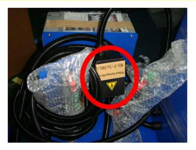
◆ Take out the electrical junction box which is packed with the UL control box.
