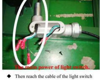
through the tube into the steel adapter box
