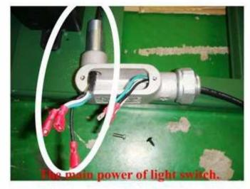
Then reach the cable of the light switch through the tube into the steel adapter box
