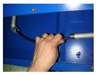
• Lock the Electrical Metallic Tube to the 45° elbow.
