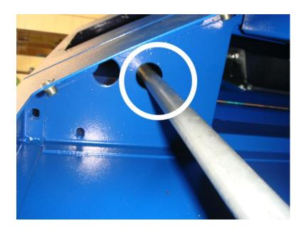
Insert the cable of the light into the Electrical Metallic Tube number: 2
