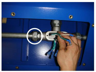
• Take out the cable from the tube and equip it into the steel adapter box.
