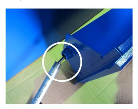
Lock the Electrical Metallic Tube number: 6 to the Hydraulic Hose Adapter, Female NPT to Female NPT.
