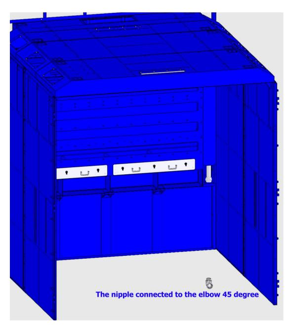
• Fasten the Nipple with the Hydraulic Hose Adapter, Female NPT to Female NPT.
