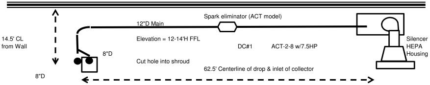
Remove fan or Cut-off saw #1 w/existing shroud; add drop into the top or rear of existing enclosure. add adapter for 8"D connection
