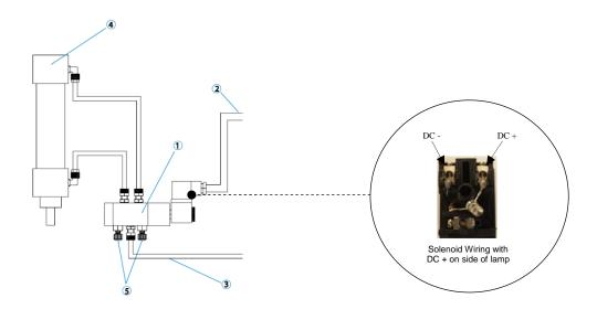
1) Solenoid Valve 2) Power Supply 3) Air Supply 4) Cylinder 5) Flux Regulators
