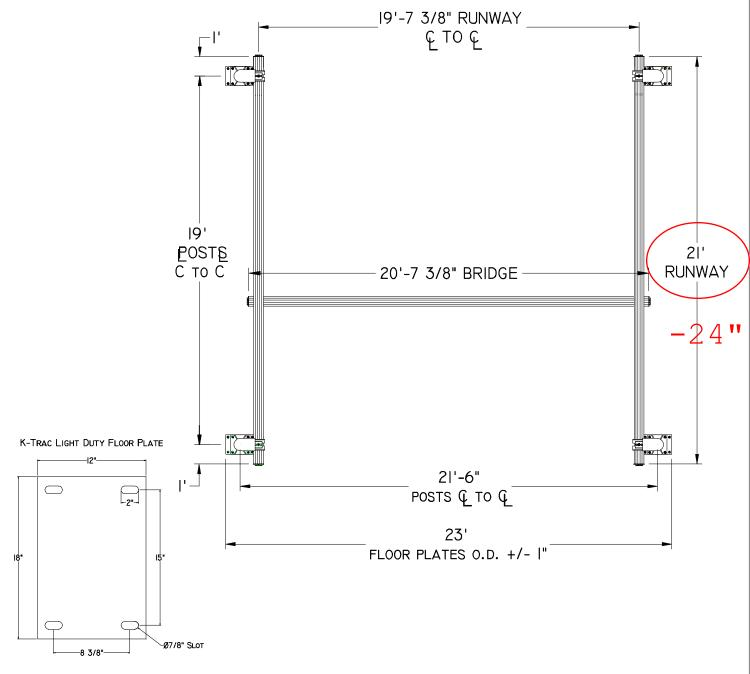
RECOMMENDED ANCHOR SIZE: 3/4" X 6" WEDGE ANCHOR
