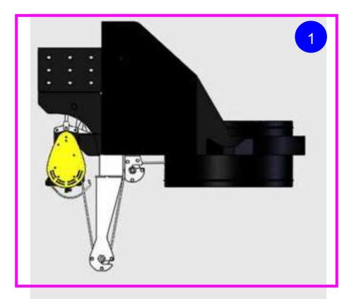
Will manufacture #1 and #2 to stimulate the situations of using the cables holding the hood and lowering it to hit something. Make sure that the cable will not come out of the wheels.
