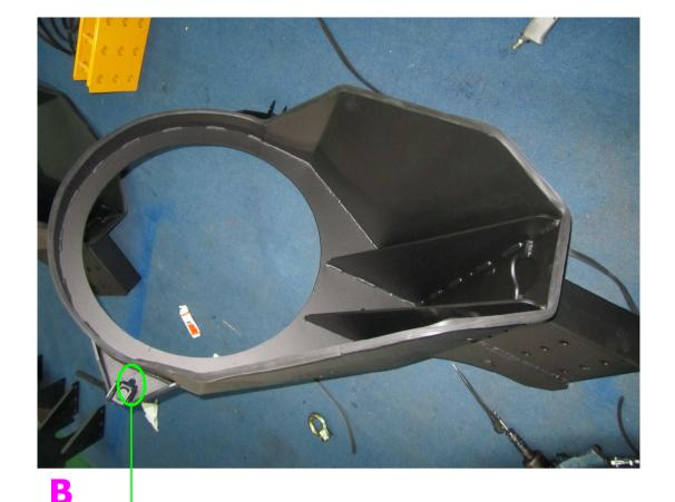
A hole pre-drilled at the bracket before shipment. Please source an eyebolt locally. Connect the carabiner with large gate opening to this eyebolt.
