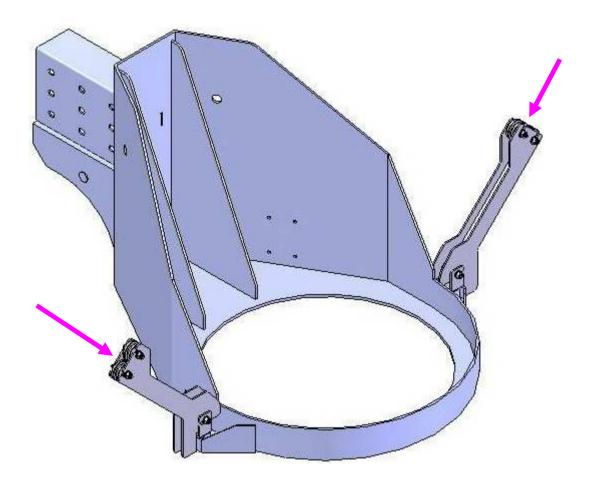
(2) additions that allow 10" space to prevent the guard (part# 162) from hitting the hood when hood travels upward and downward
