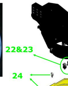
Connect the number 24 with the Flat Washer: 5/8"\*OD40\*3T, Lock Washer: 5/8" and Hex Nut: 5/8"
