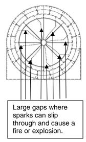
"In the past 18 months, we have had 4 fires. One fire destroyed the exterior dust collector... **We have a Blender Products Spark Cooler**... We believe we either have an issue with the Blender spark arrestor... I am looking to possibly **replace an existing "Blender" style spark arrestor** to improve the effectiveness of spark capture." Jim Jones
