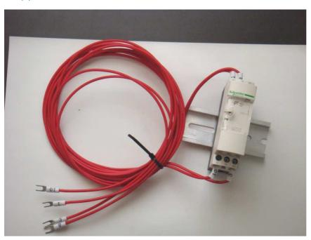
2. Install the timer near the IC board.
