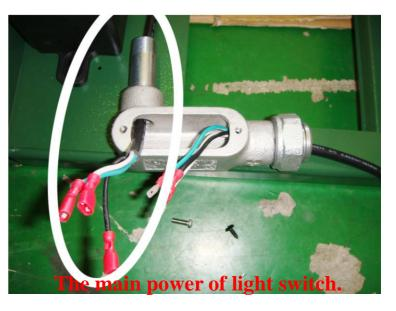
◆ Then reach the cable of the light switch through the tube into the steel adapter box
