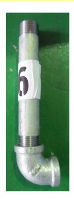
First, take out the number 6 (the tube connecting to the elbow, 90 degree.)
