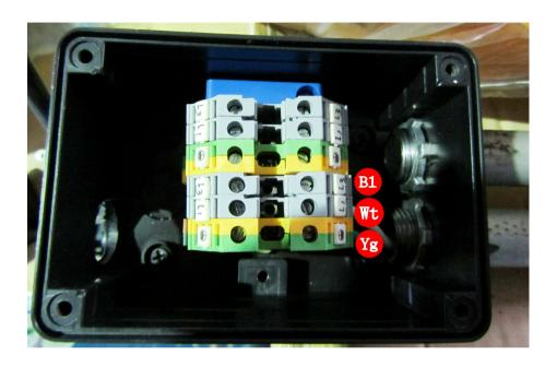
Connect the cables with the terminal blocks for the electrical junction box.
