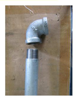
> Loosen the elbow, 90 degree.
