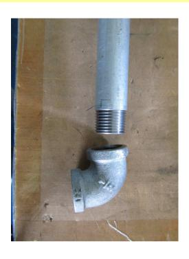
> Loosen the elbow, 90 degree.
