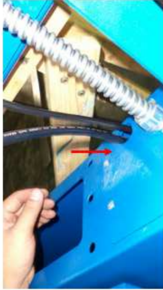
Insert the motor cable into the iron plate as arrow shown.
