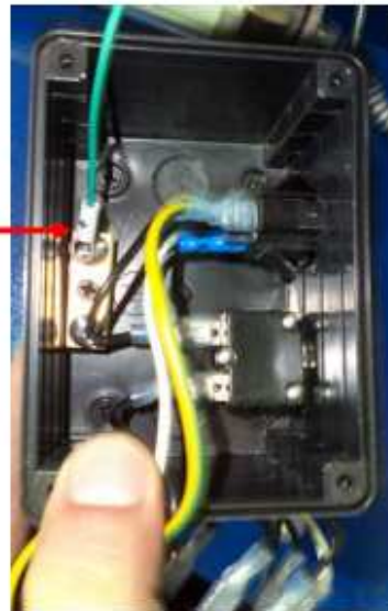
Light cable Join Green wire in here.
