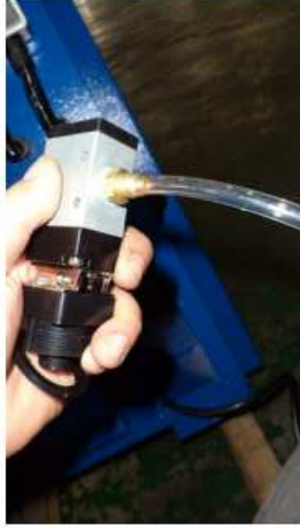
Have the PU tube installed on the copper adapter.
