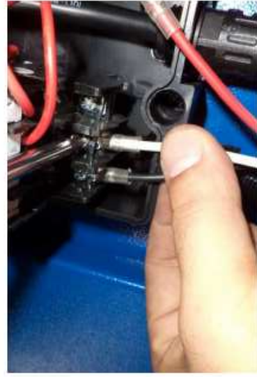
Join white and black wires onto the conjunction points.
