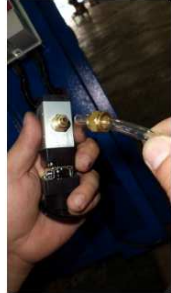
Have the PU tube installed on the copper adapter.
