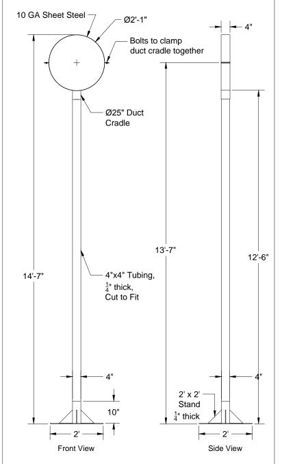
Note: Fasten to ground via 5" long anchors
