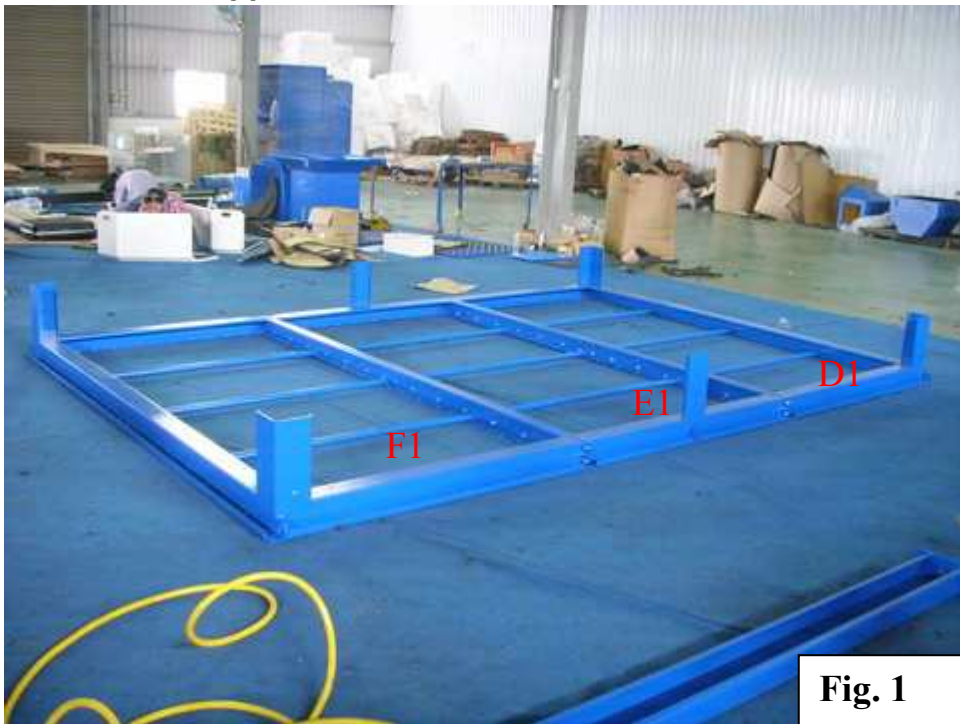
[ 1 ] Place the Frames of Hopper Section D1, E1 and E1 in order like Fig. 1.
