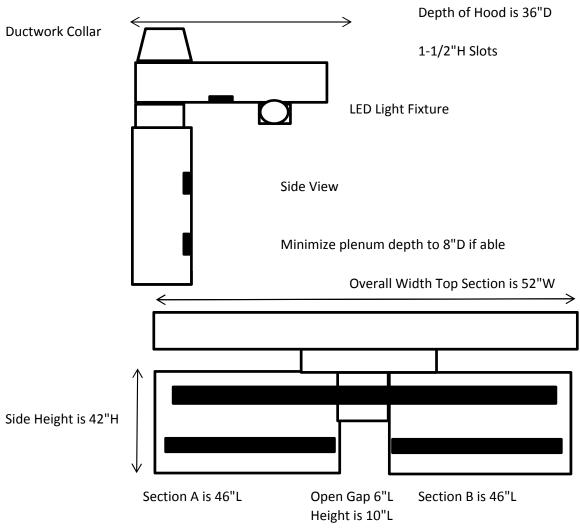
Split is necessary for welding fixture (existing)
