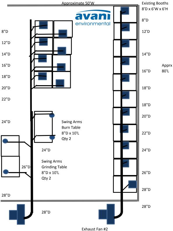
Exhaust Fan #1 Both Fans (Performance & Features) 12,000CFM @ 10"SP IN WG
