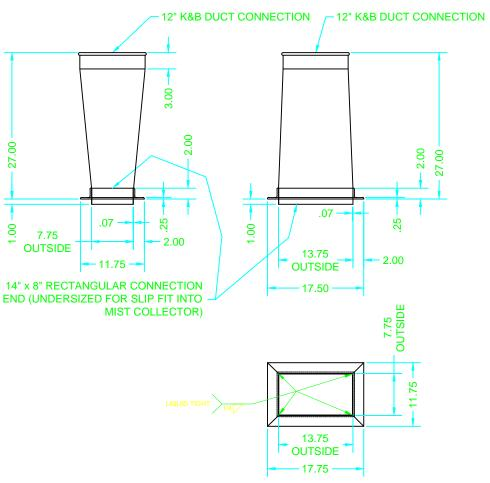
Note: All seams must be welded liquid tight
