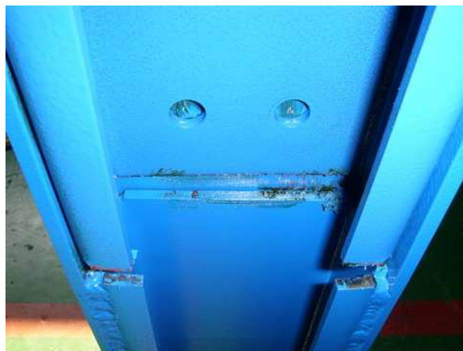
【5】 Insert the Machine Lower Section into the (3) Stands.
