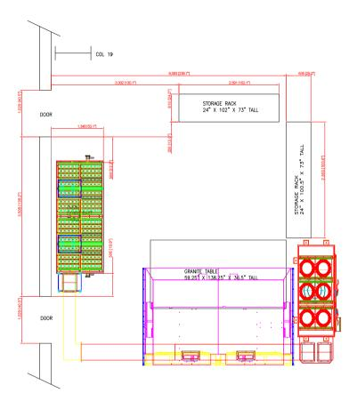
\*Add ductwork to relocate downdraft table away from door
