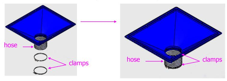
• Insert **drum Lid** into **hose** and fasten the clamp.
