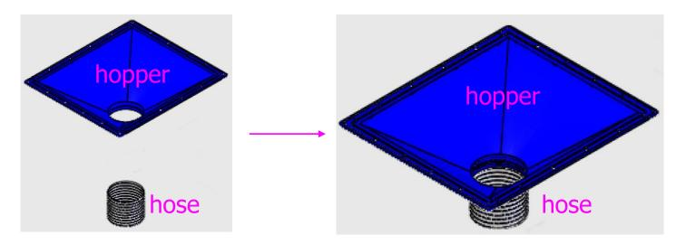
• Insert **hose** into **clamps** and fasten the clamp.
