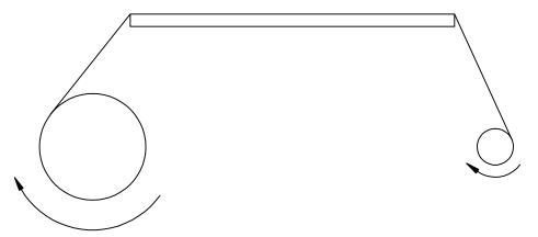
This is how the tech manual shows the roll media loaded and how it feeds and is taken up.
