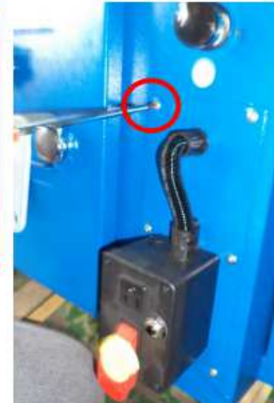
Use a screwdriver to lose the screws.
