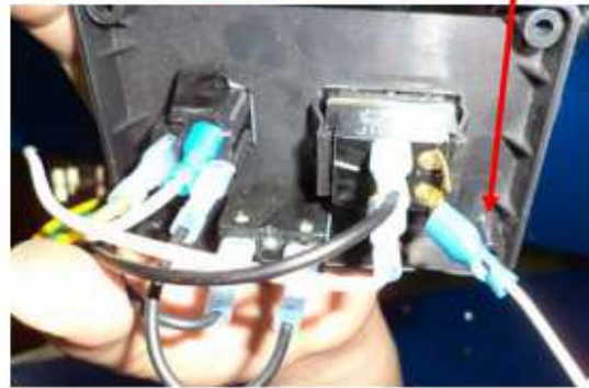
Light cable Join White wire in here.
