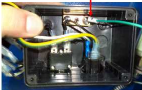
Light cable Join Green wire in here.
