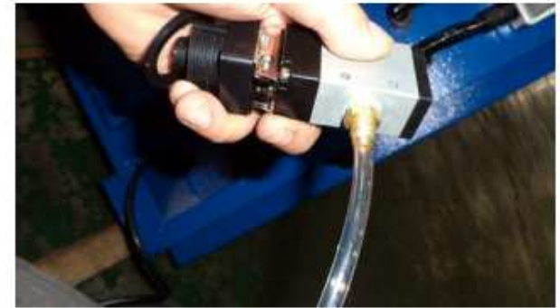
Have the PU tube installed on the copper adapter.
