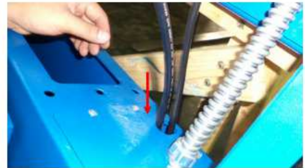
Insert the motor cable into the iron plate as arrow shown.
