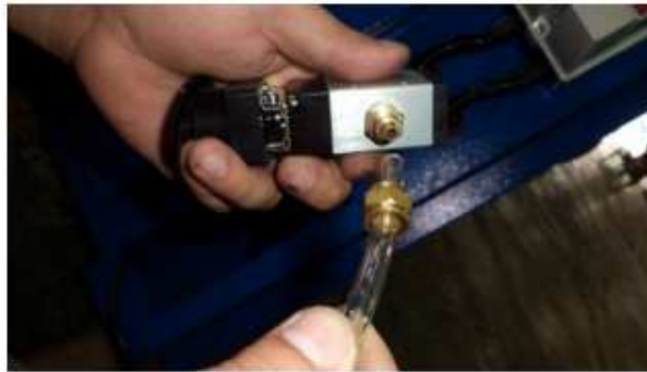
Have the PU tube installed on the copper adapter.
