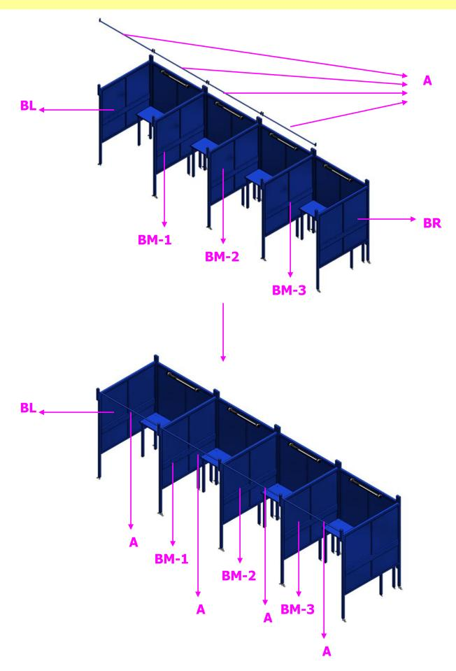
• Fasten **Sleeve Anchor** for legs to field bolted if needed.
