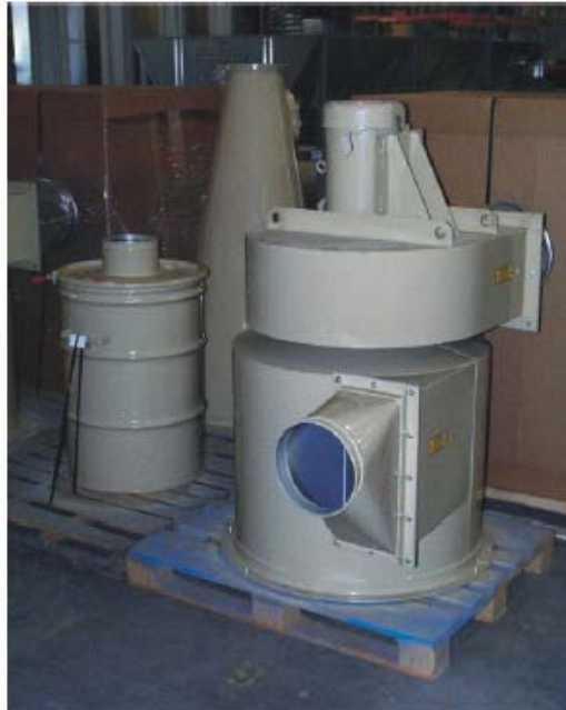
Figure 1 - Cyclone will ship unassembled in this fashion
