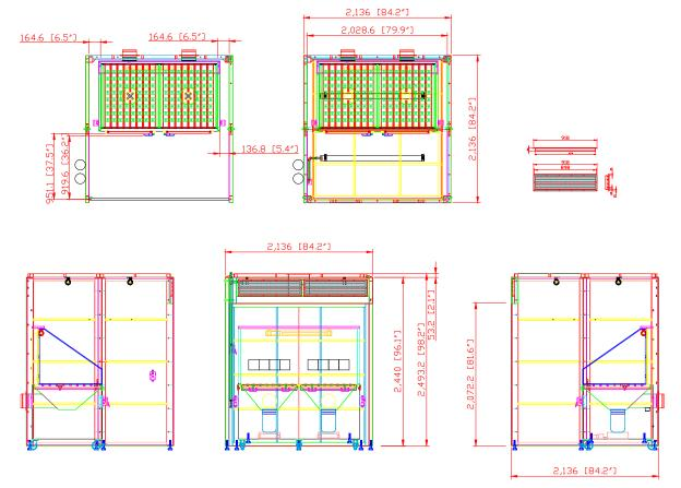
WB-7078G w/SDT-81 GRINDING BOOTH w/Downdraft table SPECIFICATIONS
