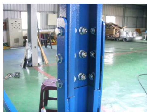
【6】 After insertion, fasten (12) pcs of 1/2''*1-1/4'' Hex Screws, (24) pcs of 1/2''*OD23*2t Flat Washers, (12) pcs of Spring Washers and 1/2'' Hex Nuts at the six locations.
