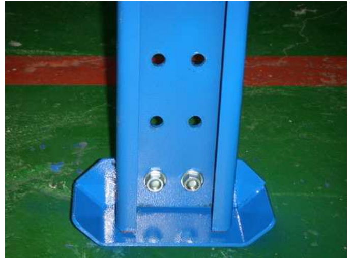
Disassemble (6) Trays under the Stands.
