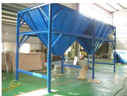
【6】 After insertion, fasten (12) pcs of 1/2''*1-1/4'' Hex Screws, (24) pcs of 1/2''*OD23*2t Flat Washers, (12) pcs of Spring Washers and 1/2'' Hex Nuts at the six locations.
