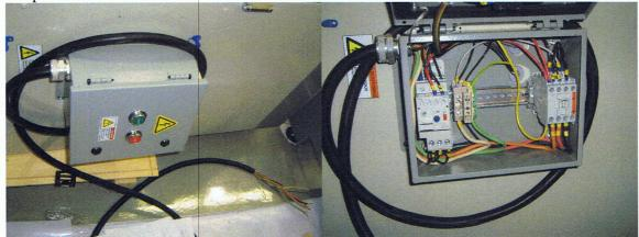
• Ensure that 15 feet of 14/5 wire is attached to the electrical box via proper strain relieves for on site connection.
