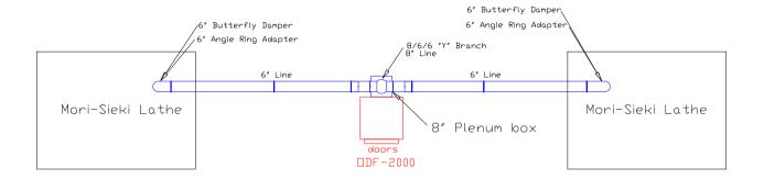
A) Each drop will have a Butterfly damper for airflow adjustment.
