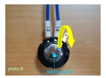
Correct installation: adjust the speed from the left to the right. Make sure that the starting point indicates to the black button (see photo C, green arrow direction, turn to point the green circle).
