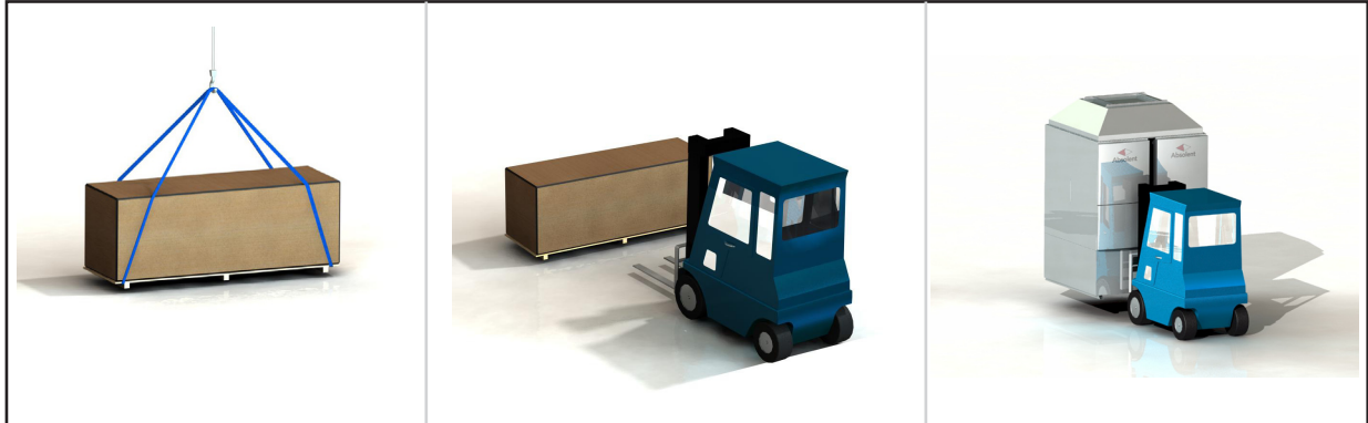
5.1.1 Lifting the filter unit on a wooden pallet with an overhead crane.
