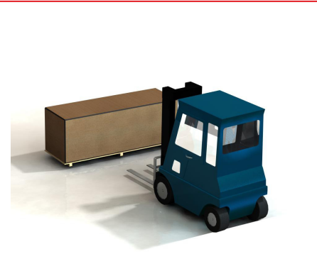
5.1.2 Lifting the filter unit on a wooden pallet with a forklift truck.
